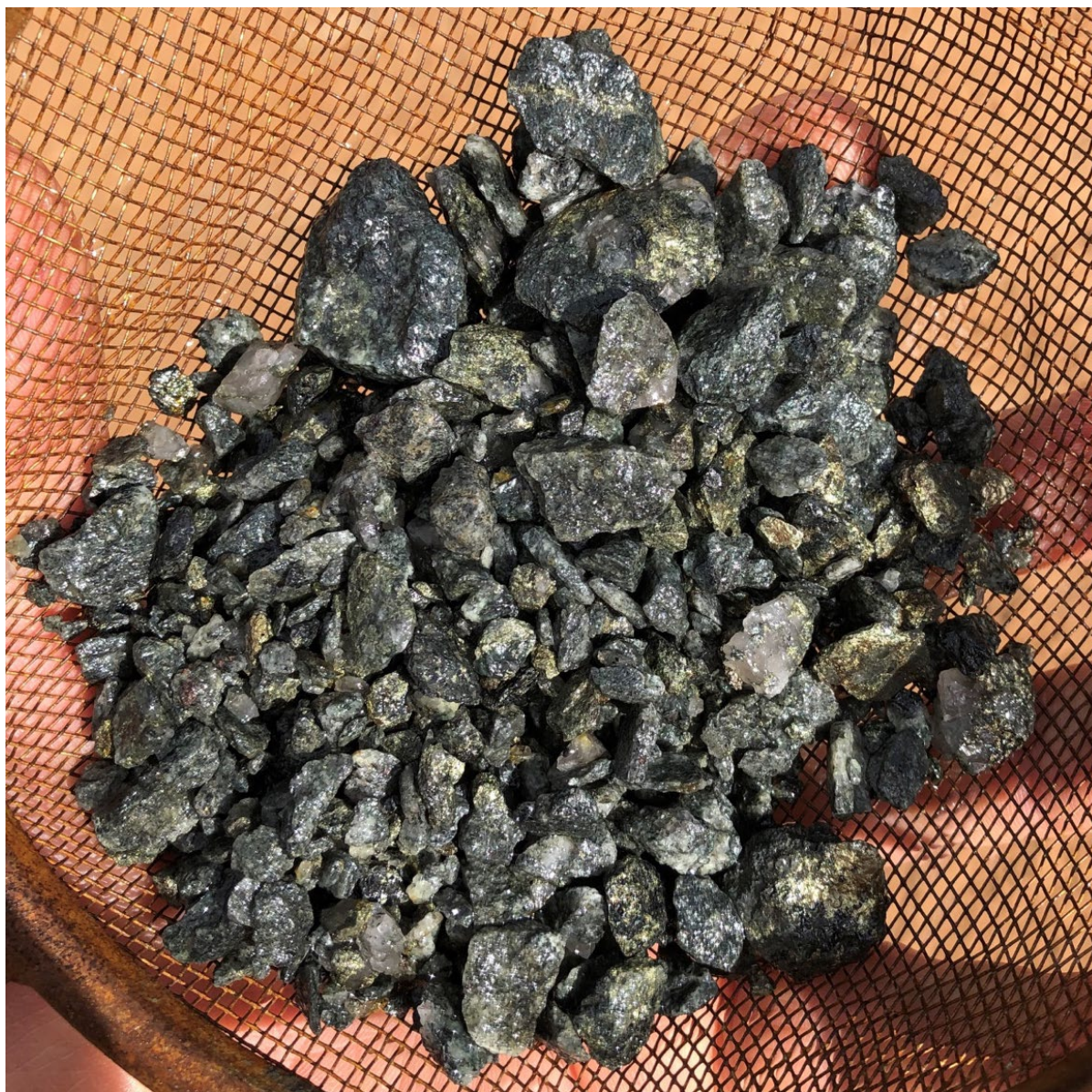
Figure 5: RC percussion drill chips from hole 21CARC119 176-177m showing chalcopyrite mineralisation. (Assays have not been received for this interval).
