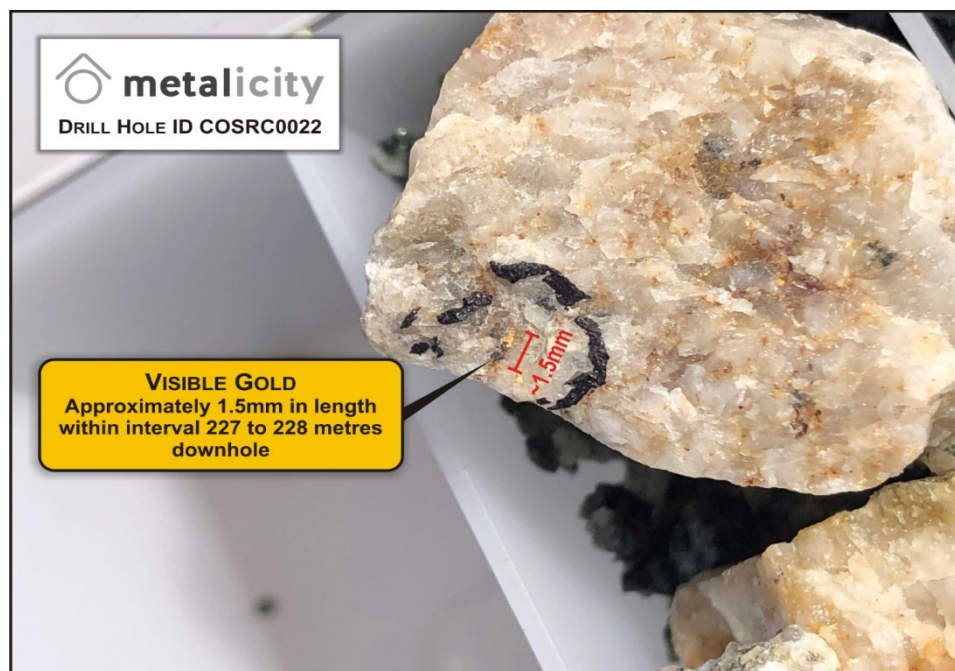
Photograph 1 – Visible gold from interval 227-228 metres in COSRC0022 at the Cosmopolitan Gold Mine.
