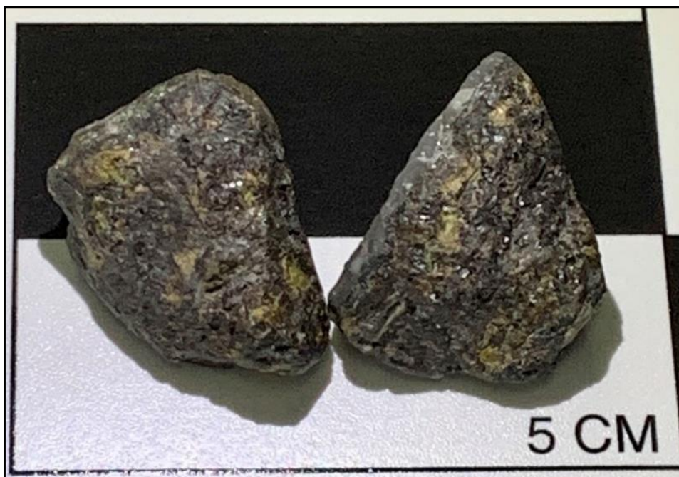
Image 1 – Massive Sphalerite (Zinc) – RC Chips – EHRC050 (80 – 81m)
