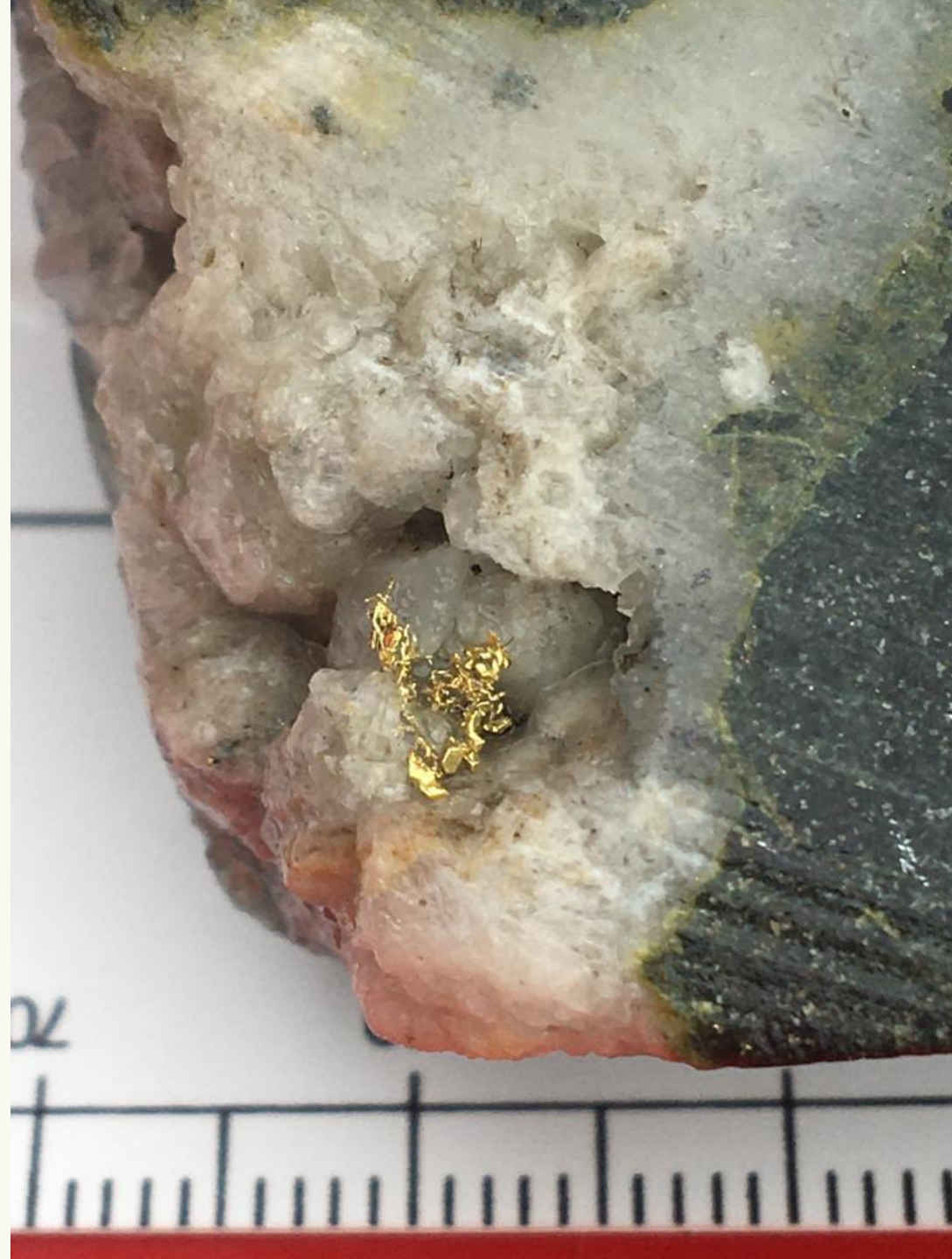
Image: QM-DH-34, 268.5m. Coarse grain dendritic gold in quartz-carbonate cement.
