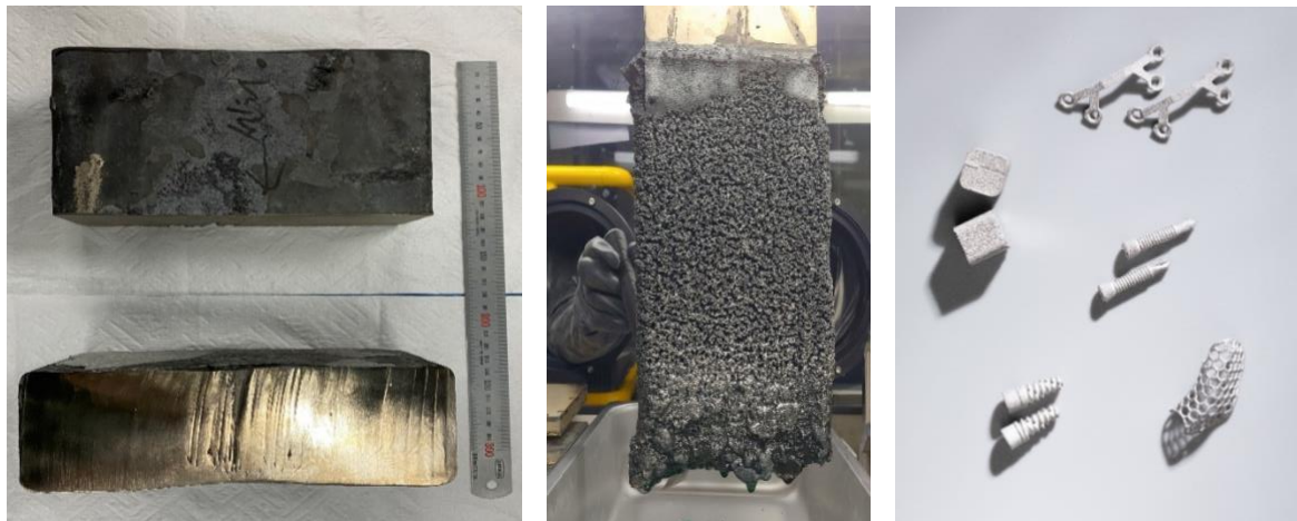
Figure 1 – a) 20kg titanium metal ingot produced by ASM, b) Creation of Ti metal powder, c) HANA AMT 3D-printed metal products
