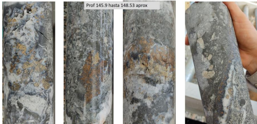
ESDD005, 147m, coarse grained sp in vein breccias; 53g/t silver + 0.76g/t gold + 3.6% zinc + 1.4% lead
