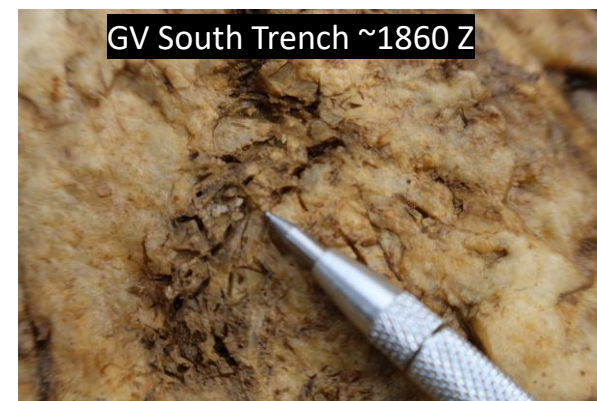
Quartz vein showing moulds and bladed textures. These textures were originally formed of carbonate and were subsequently replaced by quartz.
