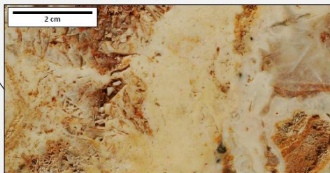
White saccharoidal (sugary) quartz vein. Note bladed carbonate texture now replaced by quartz.
