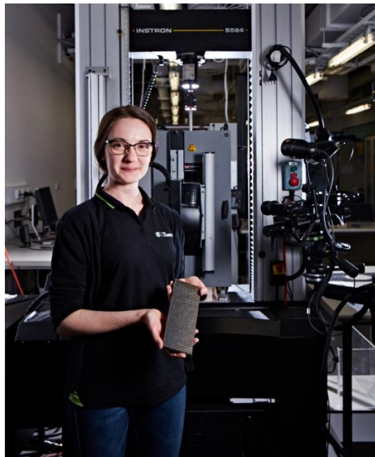
Characterising composite materials in the mechanical testing laboratory at the University of Queensland using digital image correlation to identify localised damage (Image courtesy of DMTC Limited)
