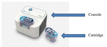
The Felix device operates on the interaction of two parts: the benchtop console and the disposable cartridges. The console consists of a docking station, for housing the cartridge, and a single button user interface. The console button initiates a fixed automated process, which optimises the final preparation of the cartridge and the supply of an electric field across the cartridge.
