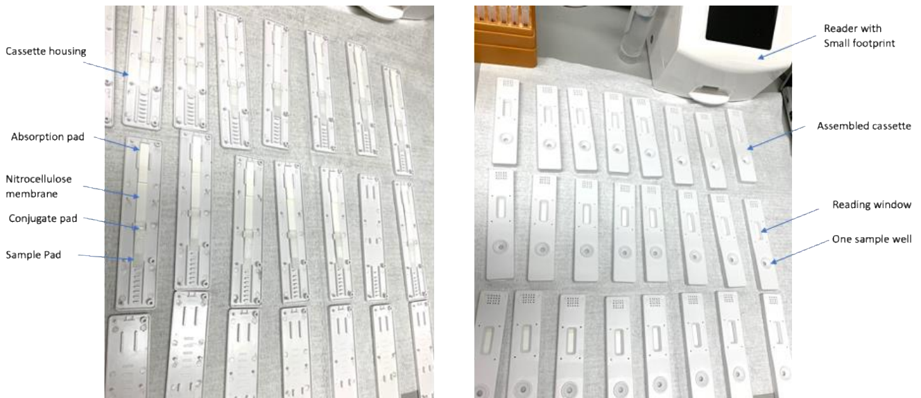
Figure 1: COVID-19 rapid test cassettes and readers being assembled
