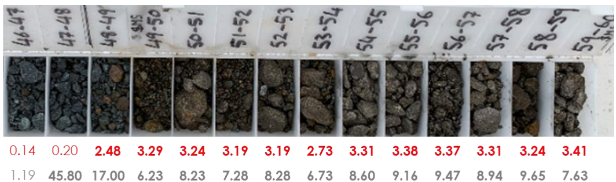
Figure 3. JRC001 drill chips and Ni+Pd assays showing the start of the massive sulphide interval from 48m.
