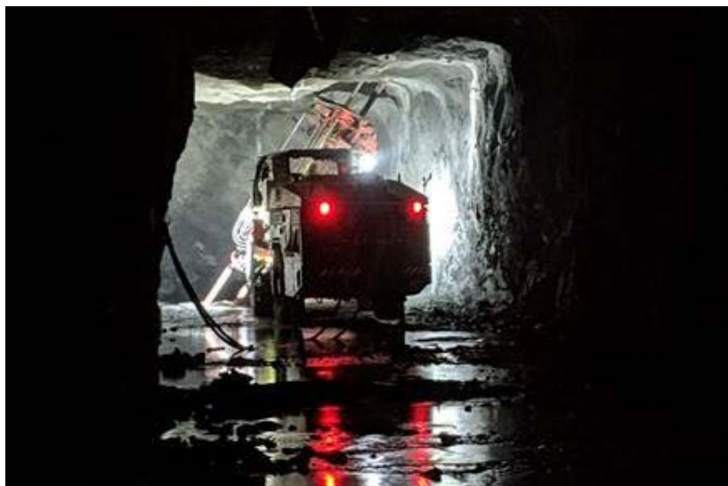
Figure 4: Automated production drill rig operating in Syama Underground Mine
