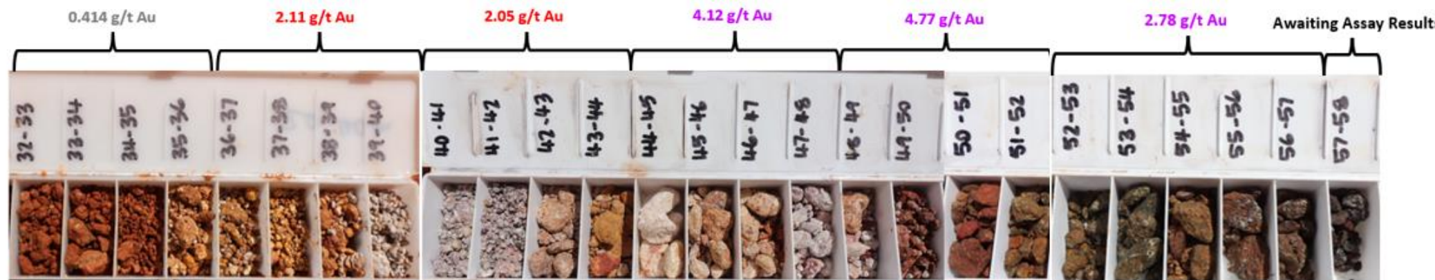
Figure 6 HEMI - BWAC258 4m composite gold assays within the strongly altered intrusion in drill chips.
