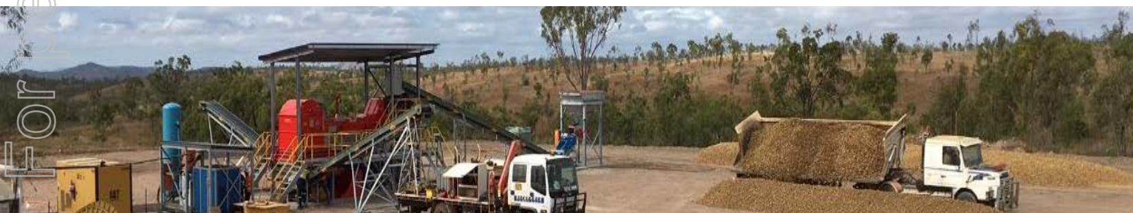
Tomra X-Ray Ore Sorter onsite at Far Fanning- ore sorting low grade stockpile material
