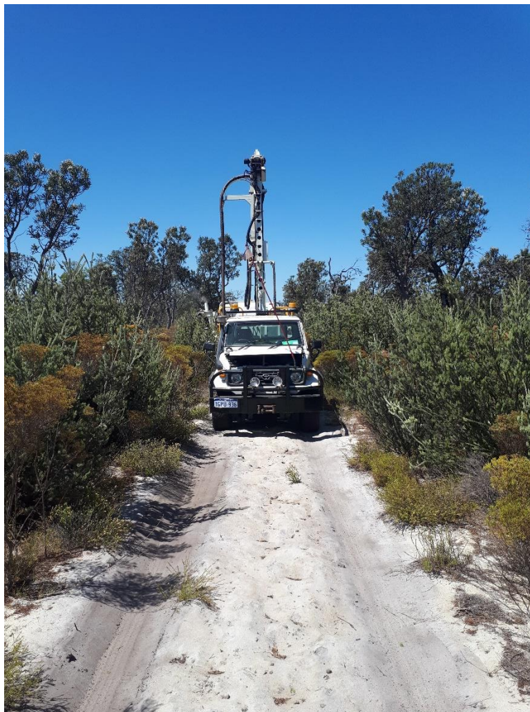
Figure 6: Landcruiser mounted Mantis 82 NQ sized aircore drill rig at Muchea
