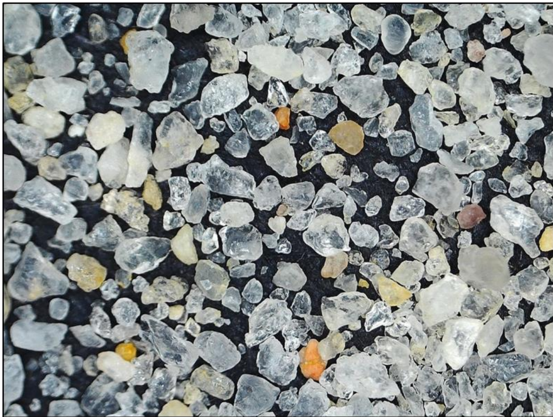
Figure 33: Muchea sand microscope picture (0.212-0.425 mm non-magnetic fraction Sphericity = 0.6 and roundness = 0.4)
