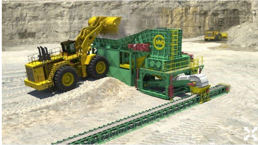
Figure 24: Mining process – silica sand loaded and screened
