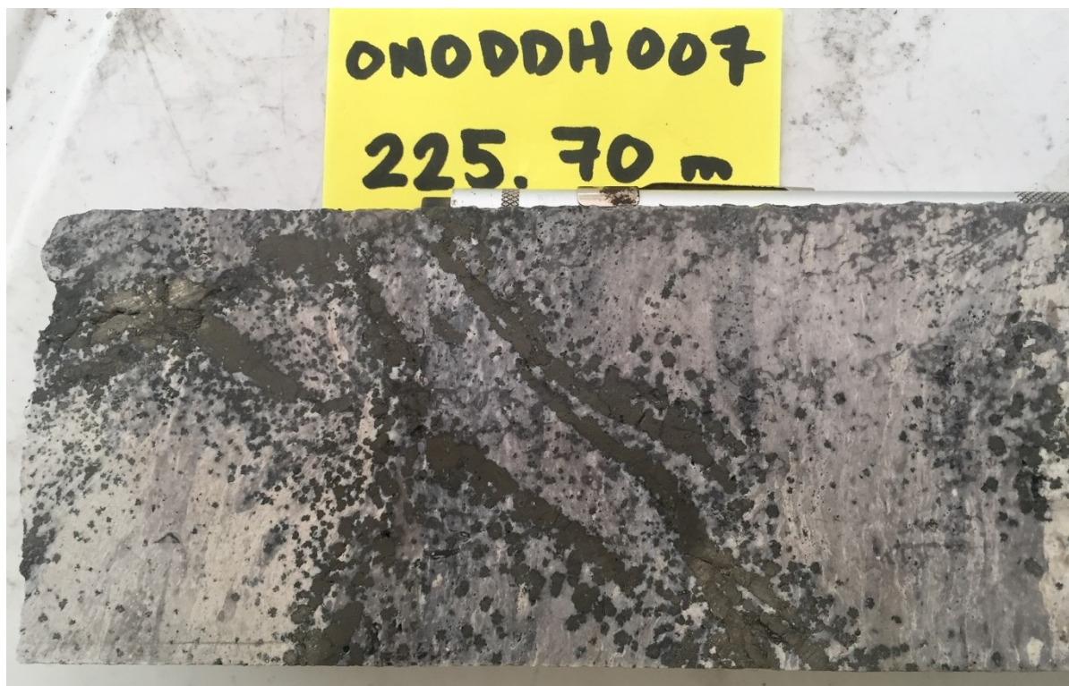
Plate 4 – Altered and mineralized volcanic host rock with up to 7% metallic sulphide in drill hole ONODDH007, HQ core from 355.5 m depth - Ono Island Project, Fiji
