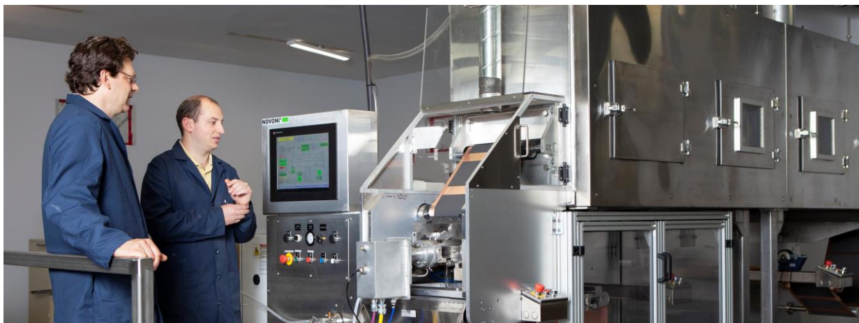
Photo: Dr Chris Burns CEO NOVONIX BTS and Professor Mark Obrovac of Dalhousie University inspecting the electrode coating line at the NOVONIX battery cell pilot line.
