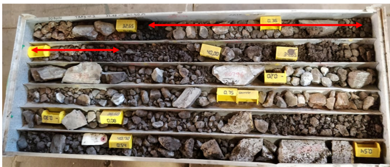
Figure 2: Diamond Drill Hole (DDBH21) "Theta Project"- Oxides drill core extremely fracture
