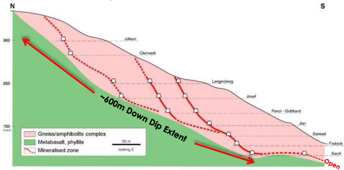
Figure 7: Section View of Josef Adit illustrating the multiple levels of adits, their respective mineralisation across three discrete veins which coalesce at depth to a single vein. Joremeny Adit is located 500m east (off section), similar level to Langenberg
