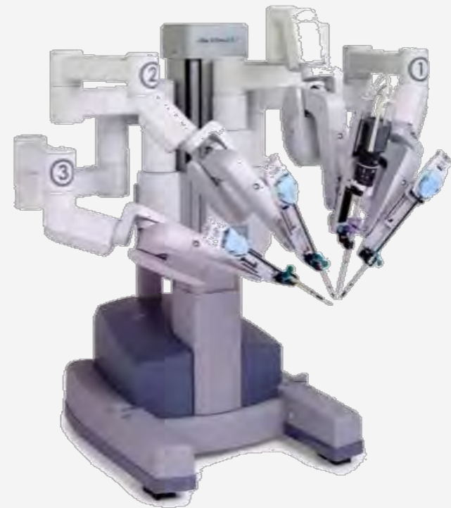
The “DaVinci” Robot (Intuitive Surgical). Systems like this incorporate intra-operative imaging of fluorescent dyes in order to better delineate tissues (nerves, vessels, tumor cells, etc.) but relatively few targeted imaging products exist at this time
