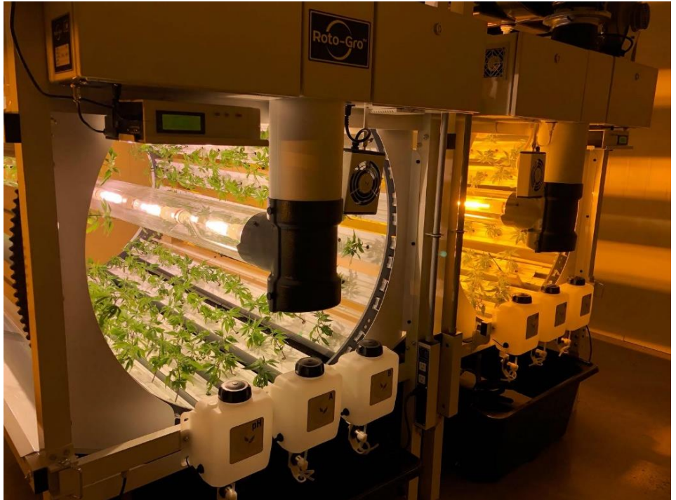
Figure 3: Testing Ceramic Metal Halide & High-Pressure Sodium Lamps
