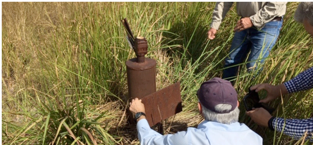
Above: Nyanda-1 well (within PL 231), drilled in 1987 prior to interest in coal seam gas in Australia encountered gas shows while drilling through coal seams. The new Nyanda-4 well will be located 50m southwest of Nyanda-1.
