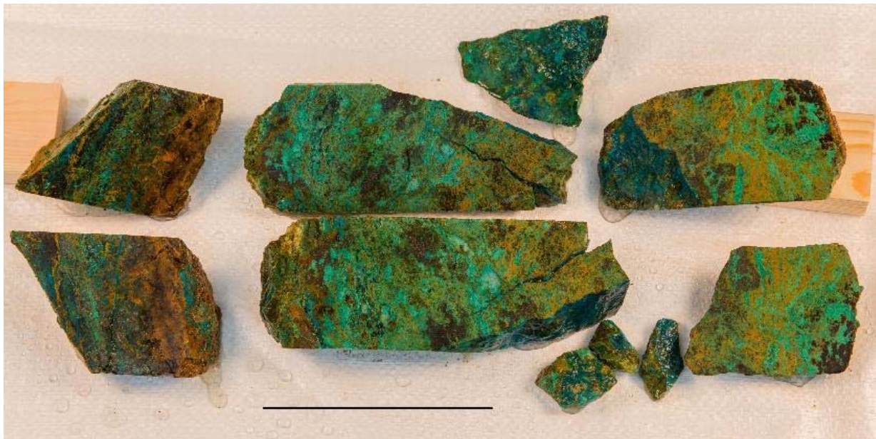
Figure 1. Visible copper oxides in hole ZX-18020, 56.7 to 57.0m down-hole depth (scale bar = 10cm). Assay for this interval 27.3% Cu, 2.5g/t Au, 82.5g/t Ag
