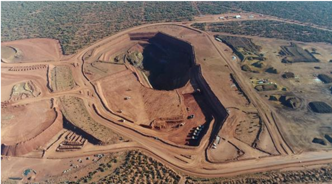
Figure 9: View looking south of the original Campaign 1 pit and the commencement of waste stripping for the Campaign 2 pit north of the original pit (November 2017).
