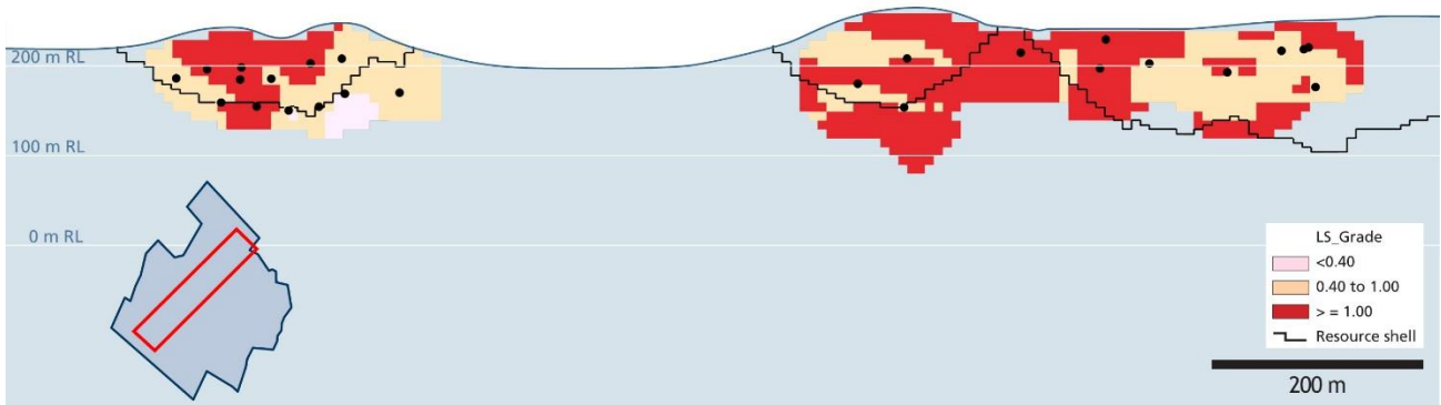
Figure 8: Schematic block long section of the S corridor looking Northwest Showing the accumulated weighted average grade (Li 2 O%) of the blocks
