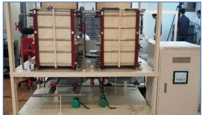
Fig 2: 2 x 10 kW VRFB-ESS
