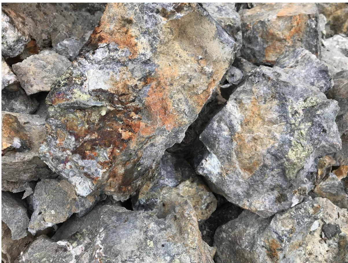
Figure 2: Stockpiled Chalcopyrite-Tetrahedrite-Erythrite Mineralisation
