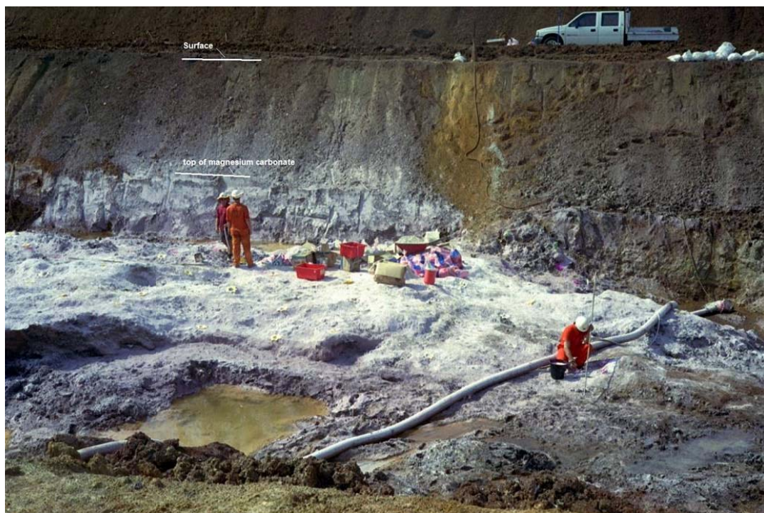
Figure 4 Test mining of magnesium carbonate rock using drill-blasting.
