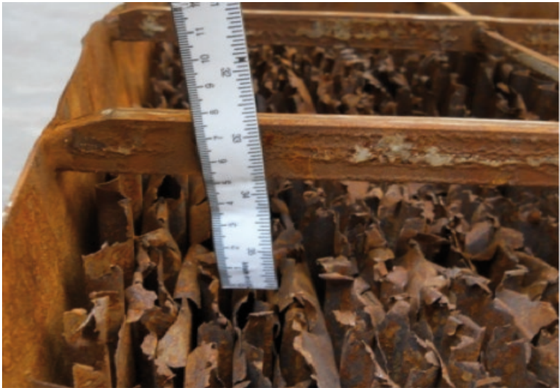
Figure 9: Example of corrosion of air heater baskets caused by bromine 1
