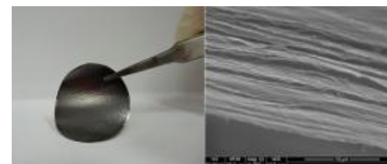
Membrane of graphene sheets from raw graphite
