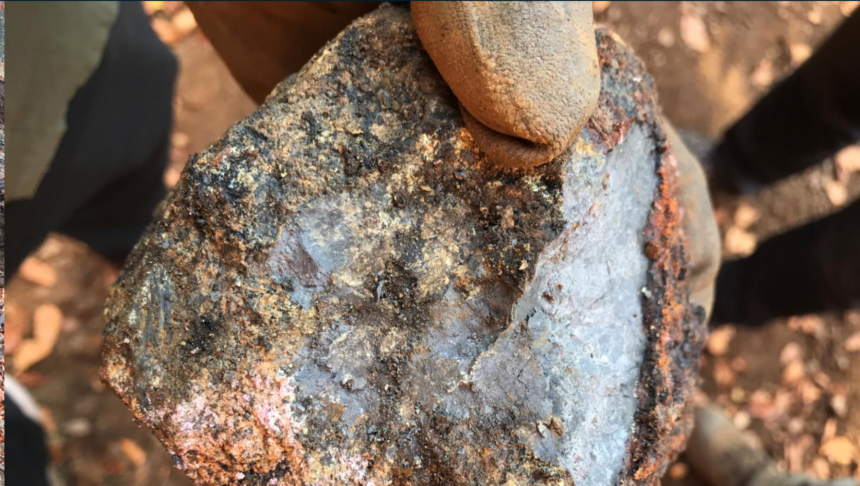
Above: Massive cobaltite-gersdorffite sulphide (Grey), Eurethrite (Pink), Annabergite (Yellow) Left: Pivo Massive Co-Ni-Cu Sulphide Zone- average thickness 70cm within broader mineralised zone of 1.5m
