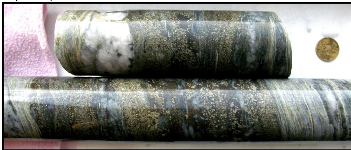
Photo 1 TIDD003: 20cm of stringer Cobalt mineralisation at 442m (almost mono-mineralic cobalt zone, likely cobaltite).
