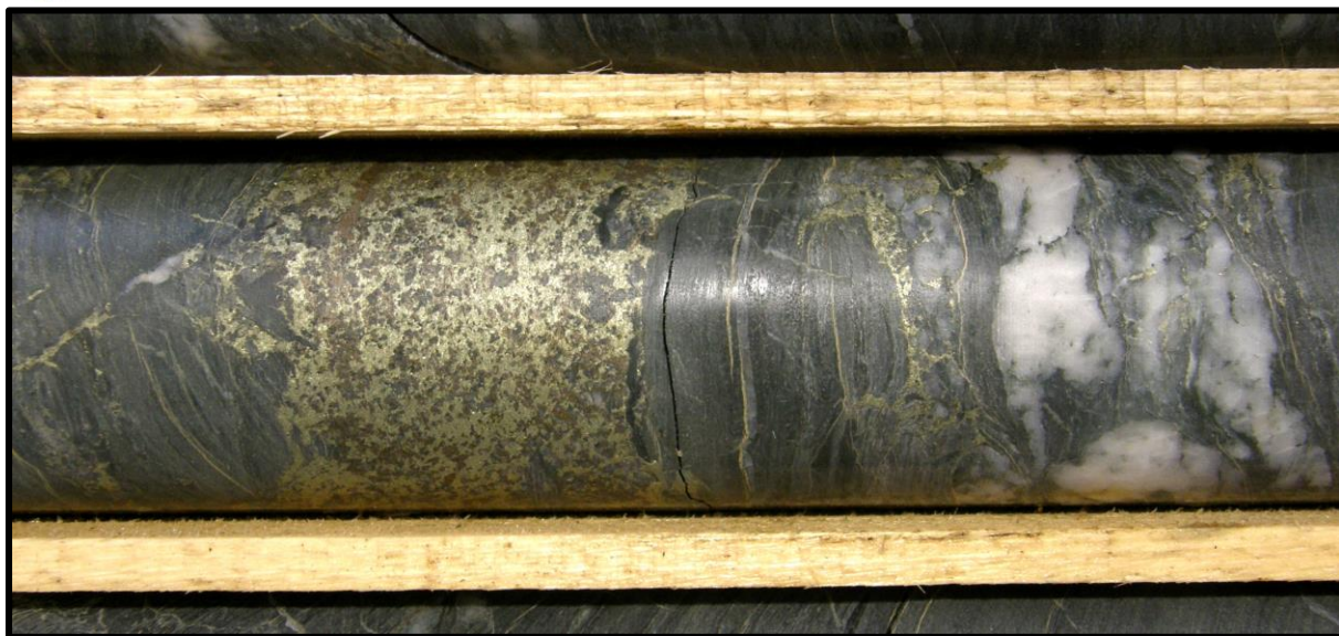
Photo 4 TIDD003 (441.7m): vein & semi massive chalcopyrite with pyrrhotite.
