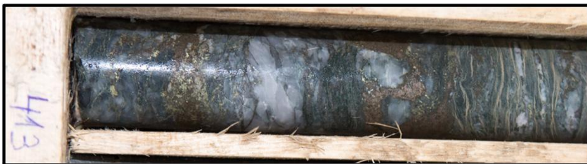
Photo 5 TIDD002 (413.0m - 413.3m): disseminated pyrrhotite, pyrite and minor chalcopyrite.
