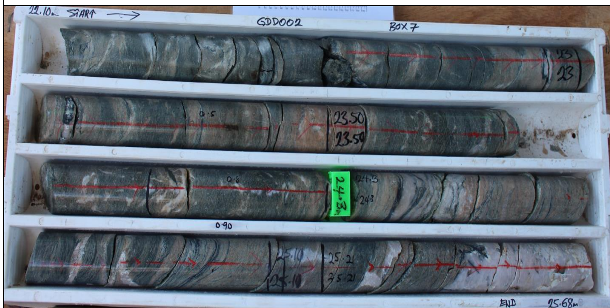
GDD002 - Tray 7, showing intense shearing, alteration and quartz – carbonate veining. Intersection 24.3 – 25.2m @ 3.66 g/t.
