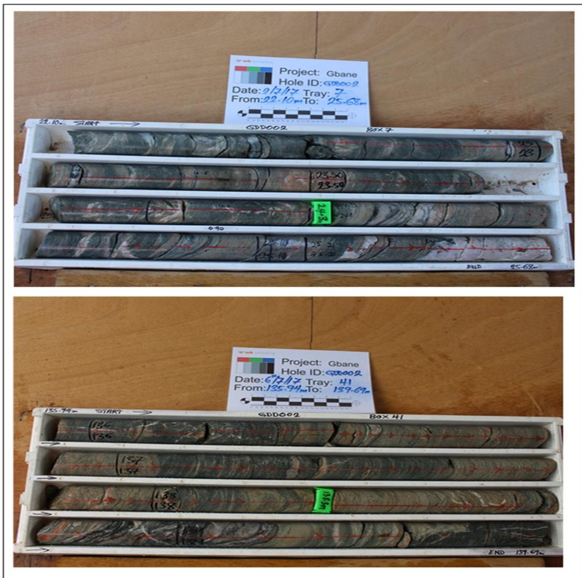
Figure 4: Core from GDD 002, showing intense shearing, alteration and quartz – carbonate veining. Intersection 24.9 to 26.3m @ 2.28 g/t and intersection 136 to 139 m @ 2.33 g/t. Intersections are typical of the main mineralised shear zone
