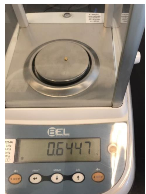
Fig.3. Gold buttons recovered from fire assay cupellation as per table 1 (see appendix 1 for higher resolution photos)
