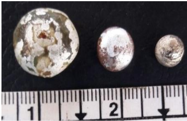
Fig. 1. Metallic buttons 1,2,3 recovered from initial smelting of 5kg Ema bulk sample
