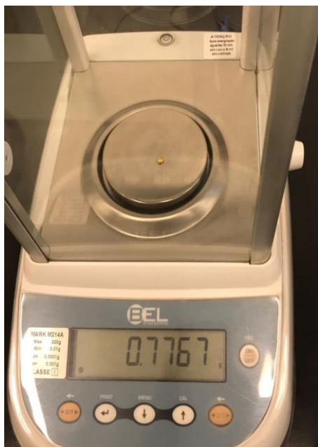
Fig.3. Gold buttons recovered from fire assay cupellation as per table 1 (see appendix 1 for higher resolution photos)
