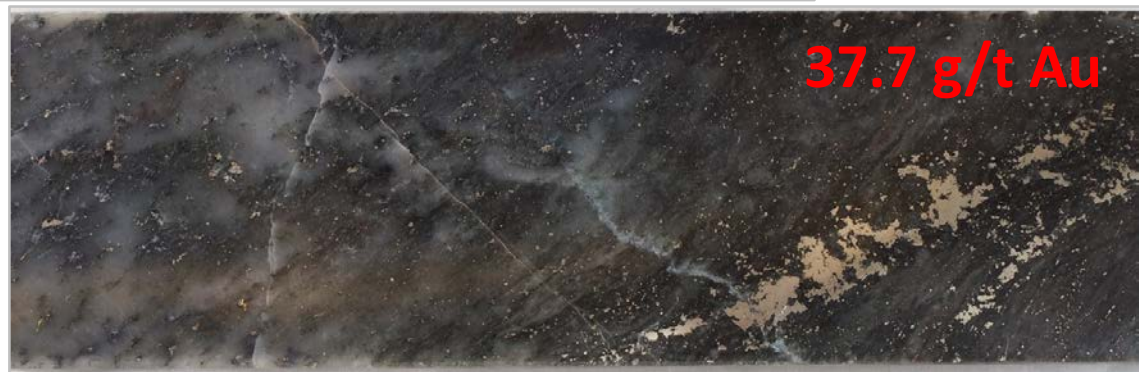
Diamond drill core photo of 17CWDD0015 at 234.36 metres downhole – part of the 37.7 g/t Au sample. Core size is NQ approximately 47.6 mm diameter and length is 17 cm
