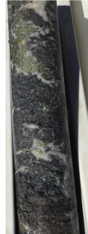
Drill core CCD02, evaporite horizon, disseminated chalcopyrite. Visible ex-gypsum crystals of evaporite horizon
