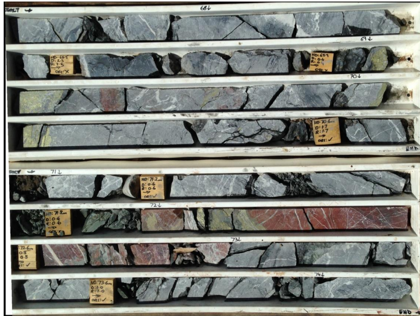
Drill core CCD03 – semi-massive chalcopyrite bands in zone of brecciation, dolomitisation, and early brick red hematite alteration, hosted by Amelia Dolomite
