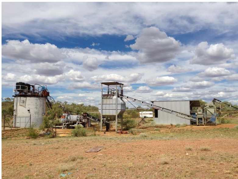
CIL Gold Plant with crushing and milling circuits at Gilded Rose
