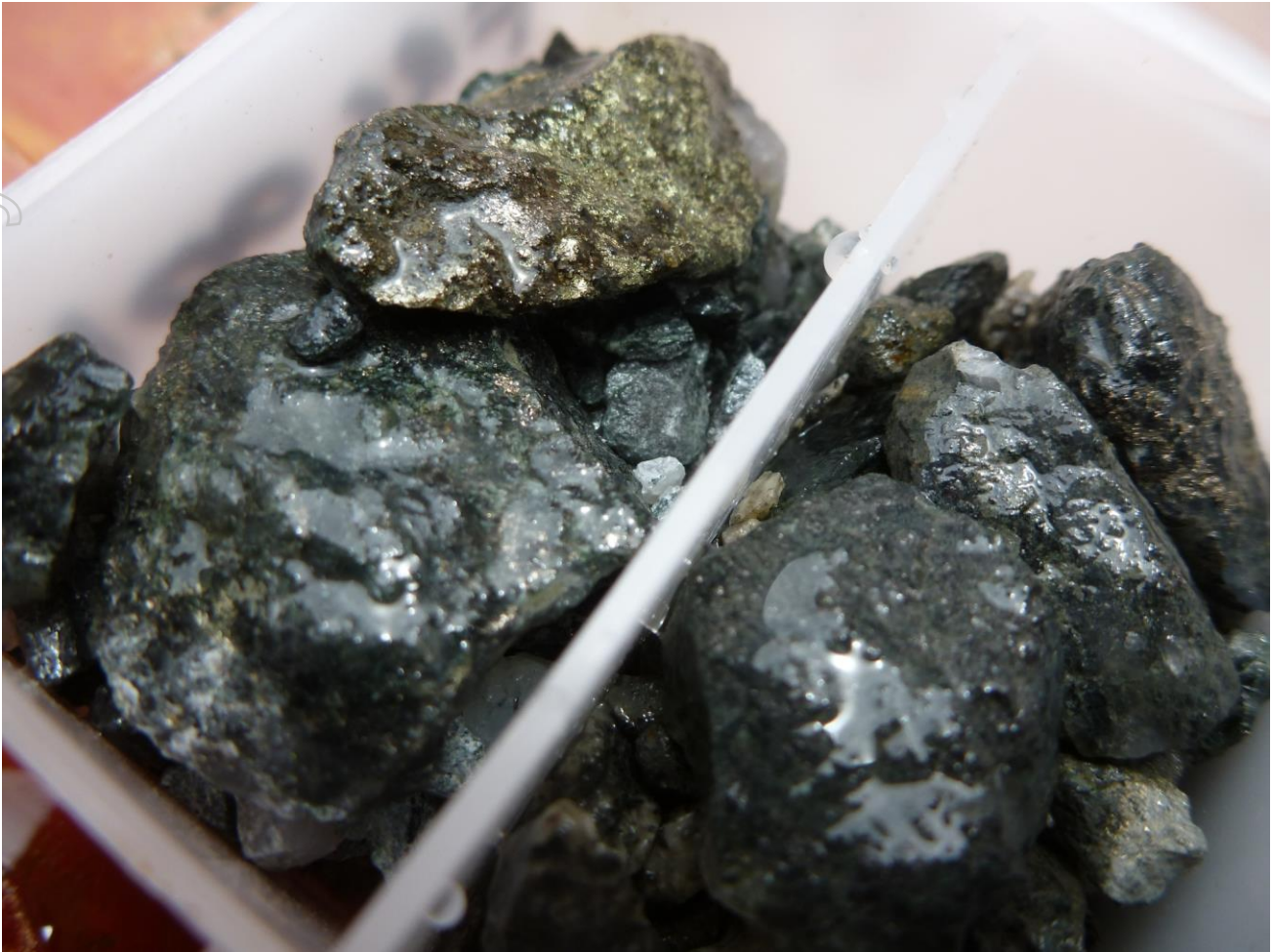
Chalcopyrite (copper sulphide) RC Chips at 221m down hole in FRC001
