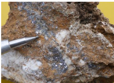
Photo 1: Mineralised vein sample. Fine matrix of sulphides (sphalerite – a zinc sulphide and galena – a lead sulphide) with Fe-oxides (red-brown) and barite (creamy white). Barite is a common gangue mineral in Zn-Ag-Pb ores in several types of deposits, especially replacement deposits, such as that at Humaspunco. Fe-oxides have developed as weathering products of sulphides and carbonates. ASSAYS PENDING
