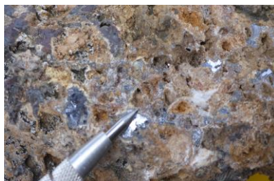
Photo 8: Mineralised float sample from a manto mine working. Highly weathered, semi-gossanous rock specimen with fine grained sphalerite and galena forming a relatively hard matrix with relatively soft clast material. The clast material is altered Jumasha Limestone which is prone to weathering. ASSAYS PENDING
