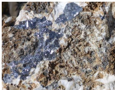
Photo 7: Mineralised manto sample from an old mine working. Very coarse galena (up to 1.0cm) and fine sphalerite with barite. The sulphides and barite here occur as matrix material in a mineralised breccia. ASSAYS PENDING
