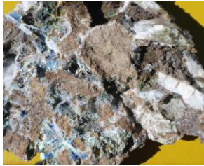
Photo 18: Vein sample located at Humaspunco West. Copper minerals in the matrix are blue-green in colour. 8.94% Zn, 560g/t Ag, 1.54% Pb
