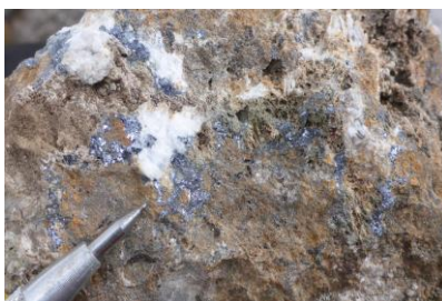
Photo 2: Mineralised manto sample. Fine matrix of sulphides (sphalerite and galena) with barite as gangue material, identified as highly altered Jumasha Limestone. ASSAYS PENDING
