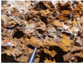
Photo 19: Highly weathered manto sample located at Humaspunco East. The very high degree of weathering at the surface has resulted in lower levels of mineralisation. The “fresh” equivalent of this manto would be expected to contain significantly higher levels of mineralisation. 0.35% Zn, 2.3g/t Ag, 417ppm Pb
