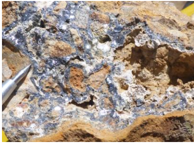
Photo 9: Similar to Photo 8 -mineralised float sample from a manto mine working. Semi-gossanous rock specimen with fine grained sphalerite and galena forming a relatively hard matrix with relatively soft clast material. The clast material is Fe-oxide rich and is partially weathered away. The resultant texture is an intricate “lattice” of sphalerite and galena.
