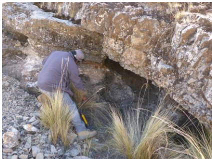
Photo 12: One of several abandoned small-scale mine workings at Pinta that had exploited manto mineralisation. The working accesses the flat lying stratabound mineralisation that characterises “manto mineralisation”. A sample was taken from this locality (Figure 1).
