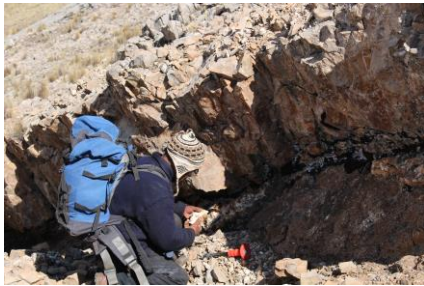
Photo 11: Manto mineralisation exposed in outcrop NW of the manto workings shown in Photo 10. The manto horizon dips at the same angle as the limestone. A sample was taken from this locality (Figure 1).
