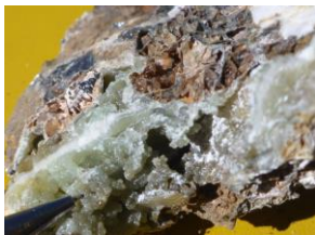
Photo 21: Vein sample located at Humaspunco West. The mineral smithsonite , a zinc carbonate, occurs as a vugh lining (pale green) where sulphides and carbonates have been “dissolved”. 20.20% Zn, 74g/t Ag, 0.65% Pb
