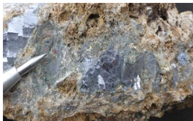
Photo 6: Mineralised vein sample from an old mine working. Very coarse galena (up to 1.3cm) and fine sphalerite with barite and calcite. ASSAYS PENDING
