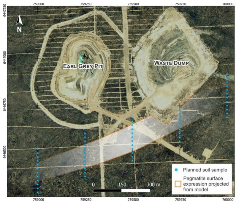
Figure 4: Surface Soil Geochemistry programme designed and underway to delineate the surface expression of the modelled pegmatite on Mining Lease M77/1080. The Earl Grey waste dump is modelled as obscuring a small portion of the surface expression of the pegmatite.
