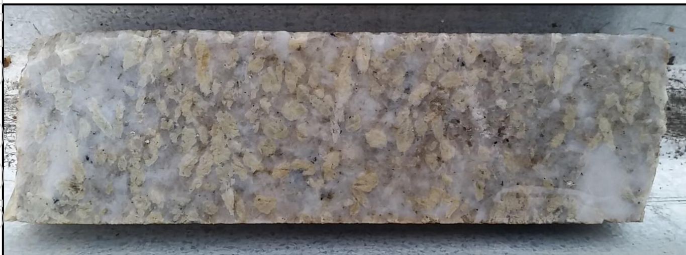
Figure 5: Spodumene crystals in a pegmatite from drill hole BUG0028 – Bounty Main results from this hole 54.2m @ 1.53% Li 2 O from 37.8m
