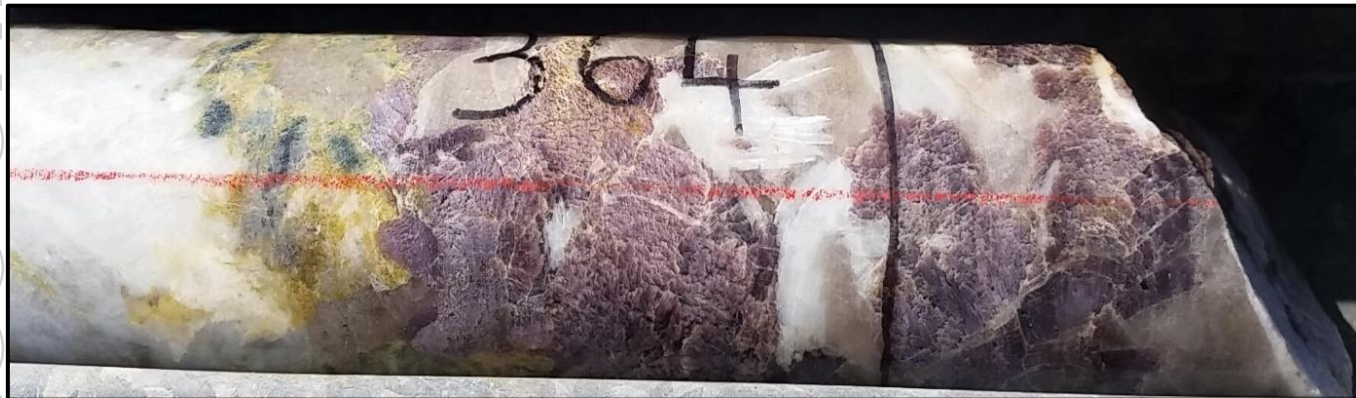
Figure 6: Multiple drill holes have encountered pegmatites rich in Lepidolite (a lithium, potassium, fluorine silicate). Lepidolite is a very soft, flaky mineral which derives its name from the Greek word for "scaly". This mineral is often a violet or purple colour but may also be shades of light green. The example of Lepidolite shown in the figure is from drill hole CBV024DT from the Blue Vein Deposit from 364m down hole.
