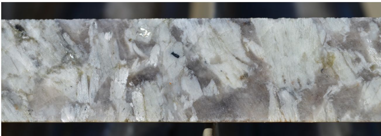
Figure 1: BUG0170 quarter core containing abundant spodumene crystals
