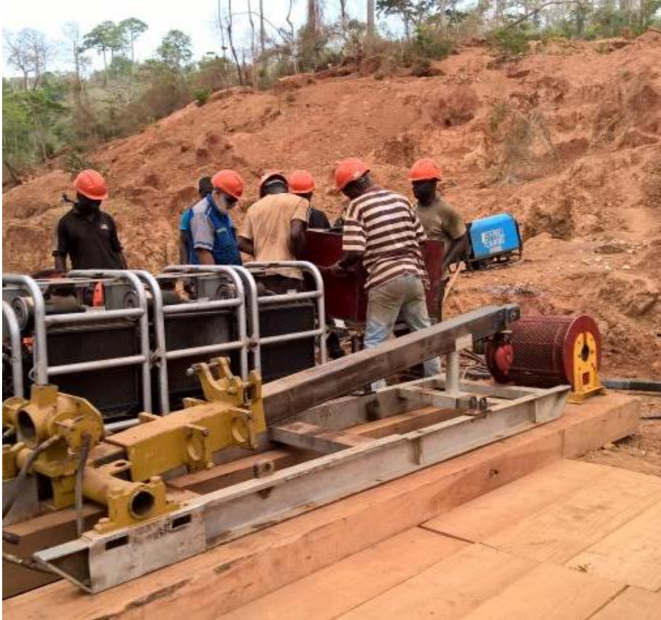
Figure 3: Portable diamond drill rig being set up on first drill site at Kokoumbo.
