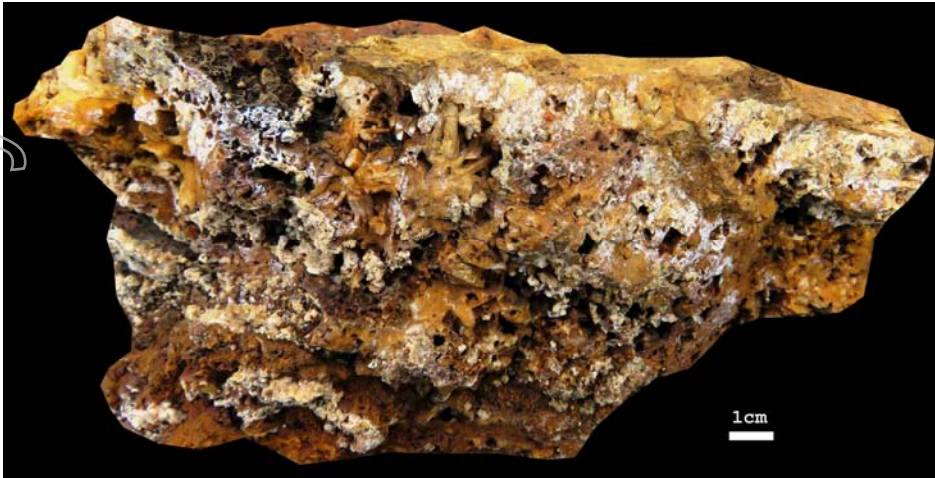
FIGURE 9: Quartz-hematite (after sulphide) vein. XR14172. 87.88g/t Au and 1.24% Cu.
