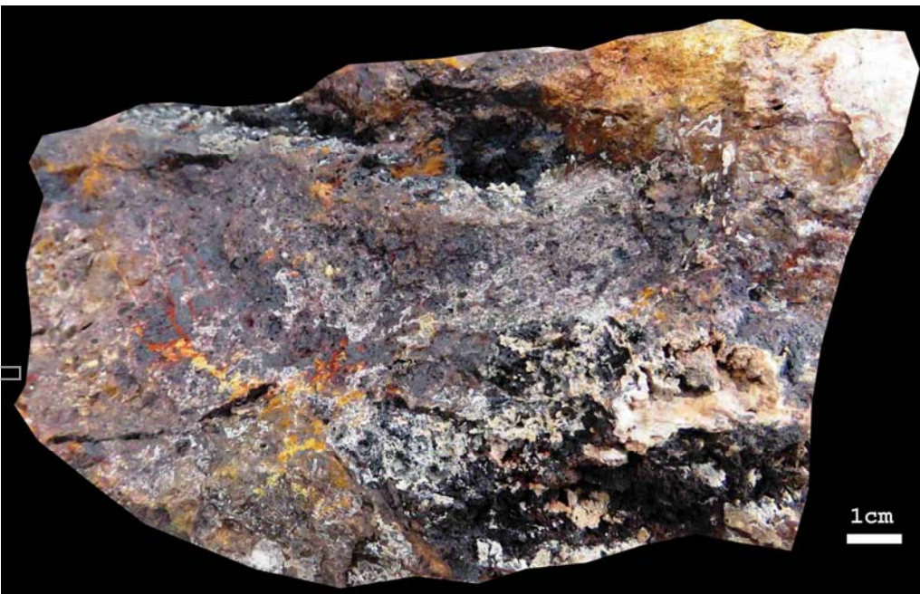
FIGURE 8: Quartz-hematite (after sulphide) vein XR14127. 56.8g/t Au and 0.41% Cu.
