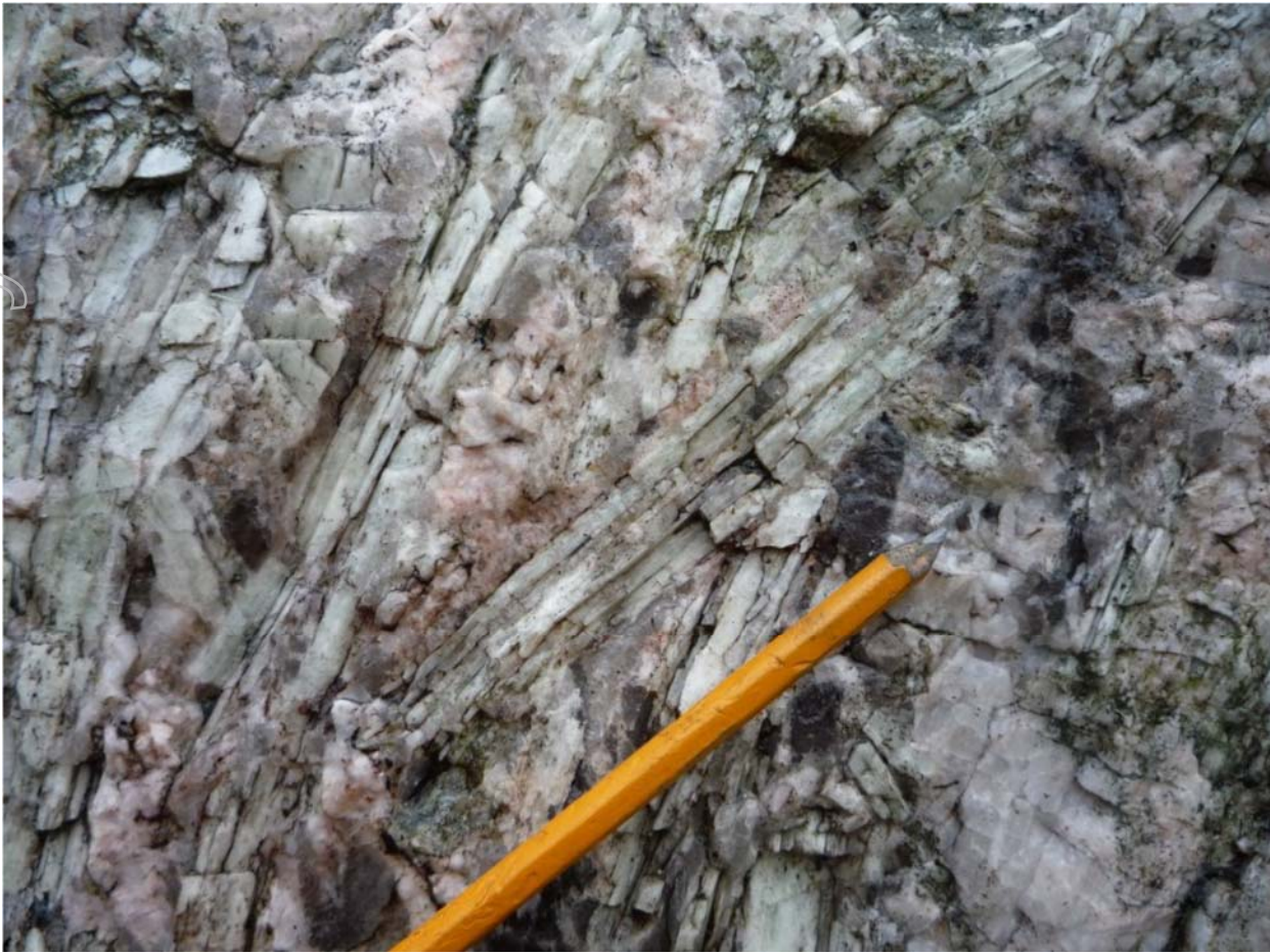
Photo 1: Light green blades of spodumene crystals interlocked with light pink to grey feldspar.
