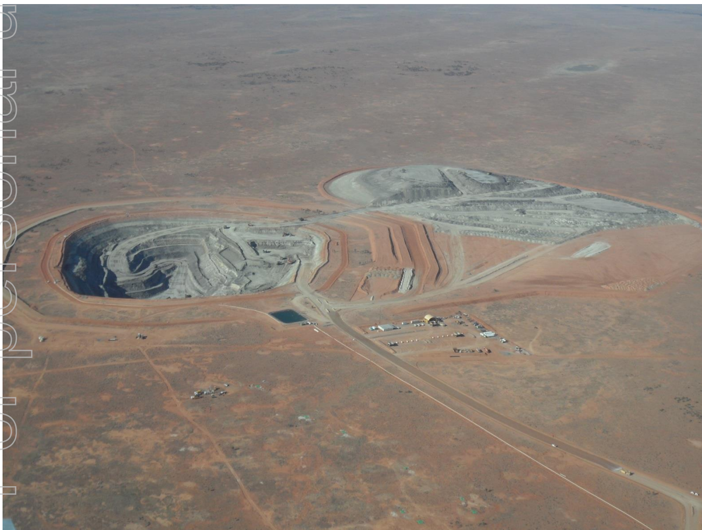
Recent aerial view of the Portia open pit and waste dump
