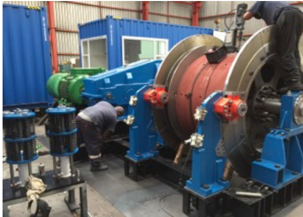
Photo 1. Main Winder undergoing inspection after trial assembly
