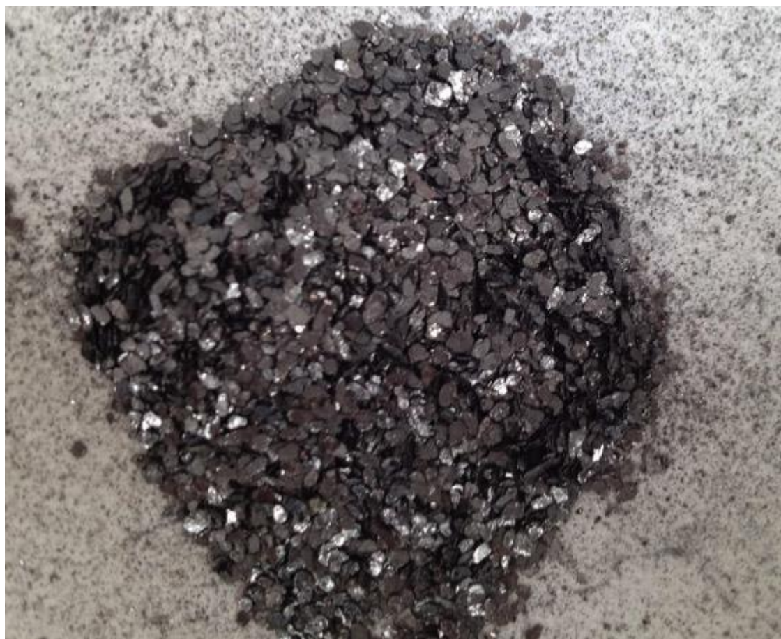
Figure 7. Super jumbo flakes (>>600µm) from diamond core hole (CRA090) at Paxtons prospect
