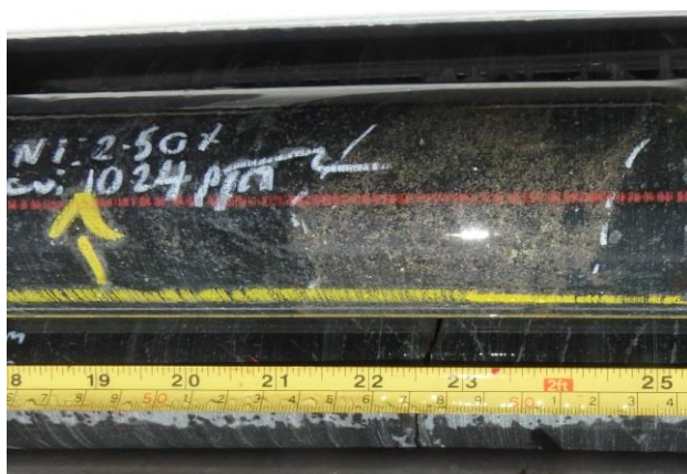
Photo 1: RHDD0027 2.5% Ni Veinlet from 186m. Photo 2: RHDD0027 7.04% Ni Blebby Sulphides from 360.5m
