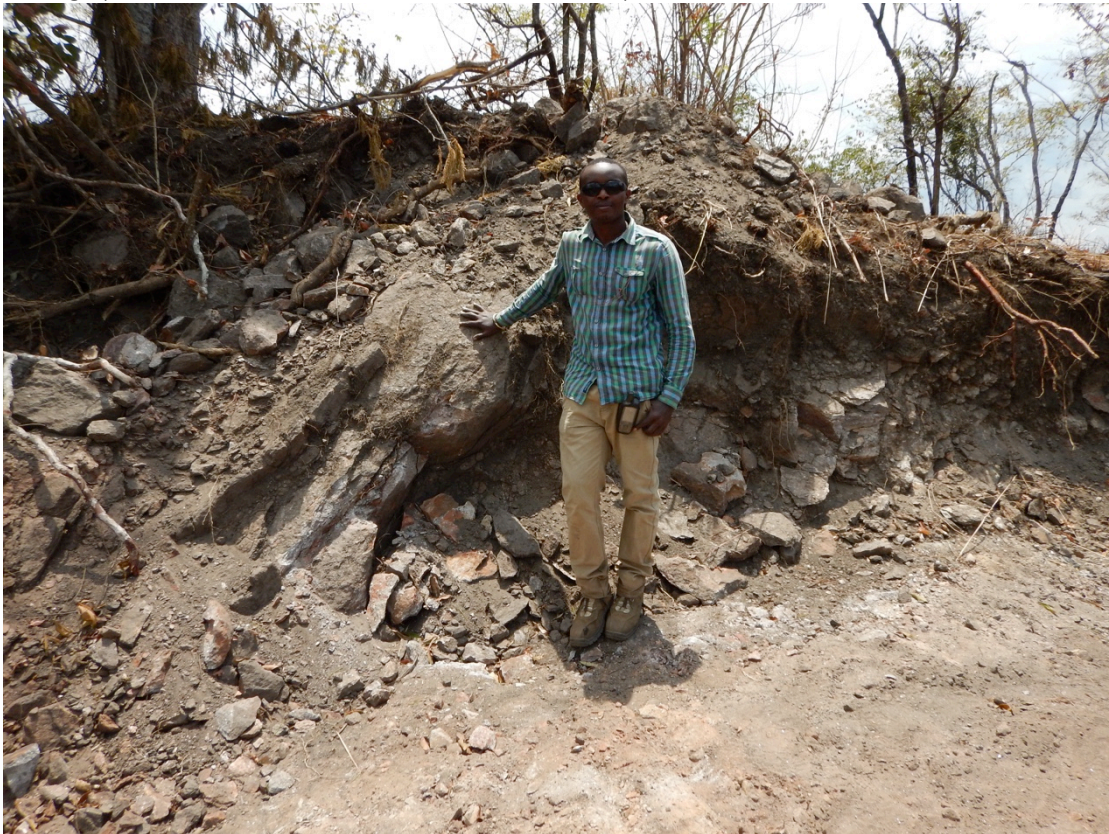
Photos 1,2. Top: Outcropping graphitic schist on Ulanzi north ridge adjacent to where the 29% TGC bulk sample was collected. Bottom: Photo of bulk sample being collected. Graphite is quite visible on surface of rocks.
