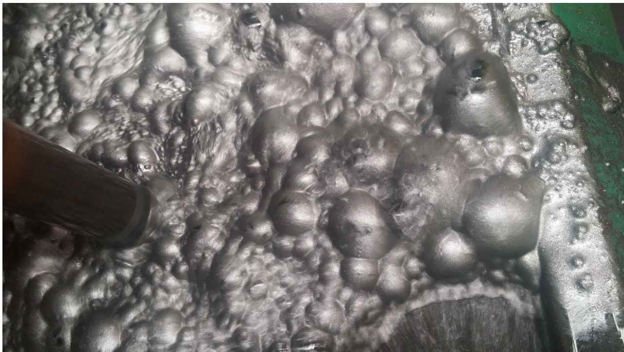
Photos 3,4. Ulanzi graphite concentrate in float cell. Final results are expected in December.
