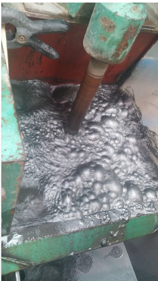
Photos 3,4. Ulanzi graphite concentrate in float cell. Final results are expected in December.
